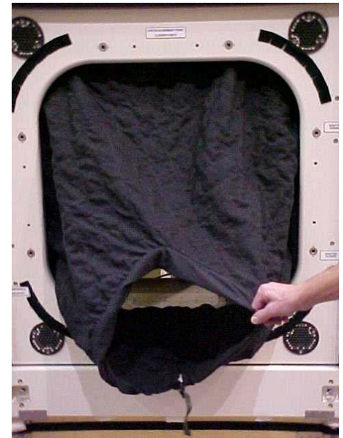
Payload Shroud Installed
