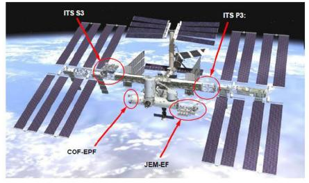
FIGURE 3.0-1 EXTERNAL PAYLOAD ATTACHMENT LOCATIONS
