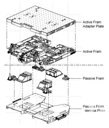
FIGURE 4.1.2-5 AFRAM AND PFRAM EXPENDED VIEW (NOTE: AFRAM ADAPTER PLATE AND THE AFRAM IS CONSIDERED A SINGLE UNIT) The Payload Mass capabilities for each ExPA, excluding support equipment (e.g., ExPA/AFRAM, FRGF, electrical connector, handrails, etc.) are specified in Table 4.1.2-1, Allowable Mass and C.G. Location of ExPA Payloads, based upon the payload C.G. location.
