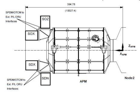
FIGURE 4.3-5 APM WITH EXTERNAL PAYLOADS AND OTCM LOCATIONS
