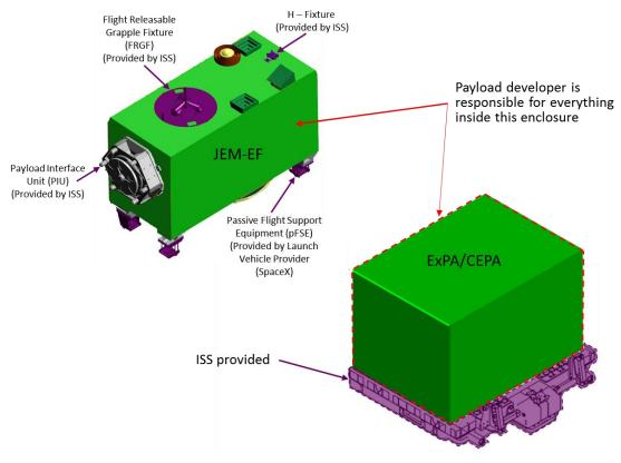
FIGURE 9.0-1 PD-PROVIDED HARDWARE INTERFACE PLANE
