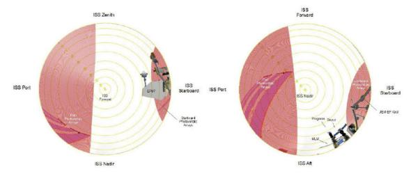
FIGURE 4.2.7-14 JEM-EF EFU9 PAYLOAD ACCOMMODATION FORWARD (RAM) AND NADIR)
