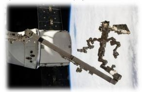
FIGURE 3.1.9 DEXTRE REMOVES PAYLOAD FROM DRAGON
