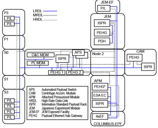
FIGURE 3.0-3 ISS C&DH ARCHITECTURE DIAGRAM
