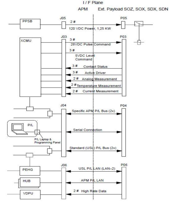
FIGURE 4.3.4-1 INTEGRATED EXTERNAL PAYLOAD SYSTEM INTERFACES
