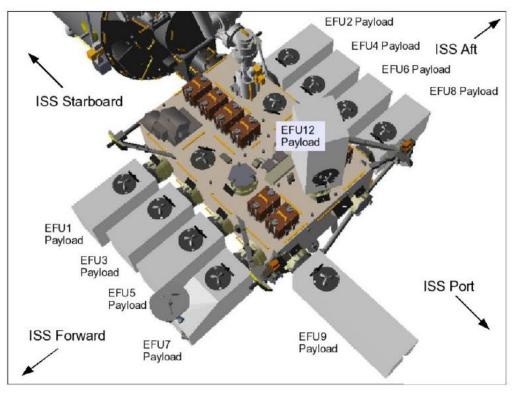
FIGURE 4.2.7-2 JEM-EF PAYLOAD VOLUME LOCATIONS AND ORIENTATIONS
