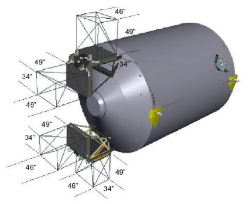
FIGURE 4.3.7-2 COLUMBUS-EPF PAYLOAD DIMENSIONS
