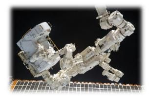
FIGURE 3.1.1-10 DEXTRE CARRIES PAYLOAD TO SITE
