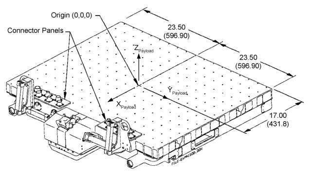
FIGURE 4.1.2-4 GENERIC EXPA PAYLOAD COORDINATE SYSTEM
