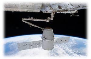
**5.** Berthing: Dragon berthing to ISS carrying Payload on Cargo Rack in Dragon Trunk.
