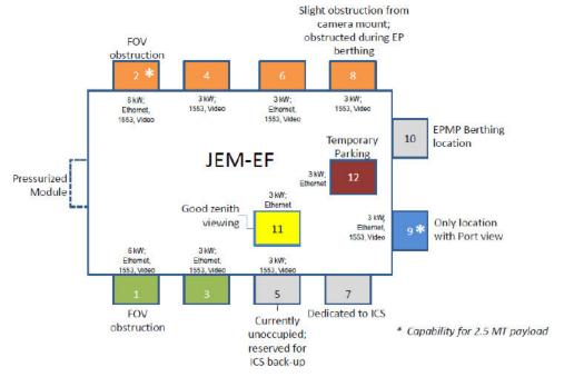
FIGURE 4.2.1-1 ILLUSTRATED JEM-EF 10 LOCATIONS FOR EXPERIMENTAL PAYLOADS
