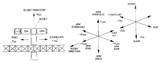
FIGURE 4.3-3 APM/ISS REFERENCE COORDINATE SYSTEM
