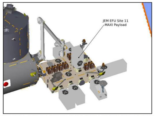
FIGURE 4.2.7-3 JEM-EF EFU PAYLOAD VOLUME LOCATIONS AND ORIENTATION
