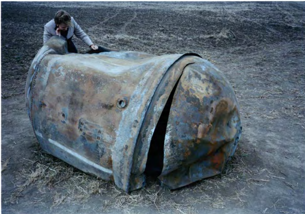
Figure 4.8-2. Fuel tank orbital debris from Delta II second stage that landed near Georgetown, TX in January 1999
